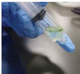
Fig. 3 - Creating vacuum in the plunger.
